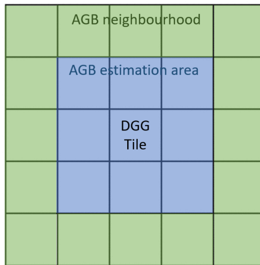
Fig.11 (top) L2b Processor, L2b AGB Processing task interfaces; (bottom) Graphical representation of DGG tiles, explaining “chromatic” input and output data selection policies.
