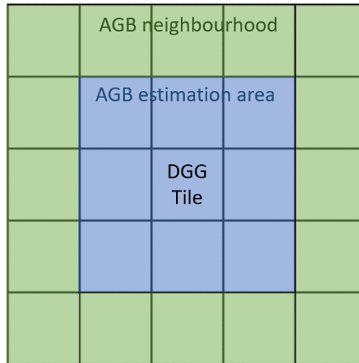
Fig.12 (top) L2b AGB Processor interfaces; (bottom) Graphical representation of DGG tiles, explaining “chromatic” input and output data selection policies.
